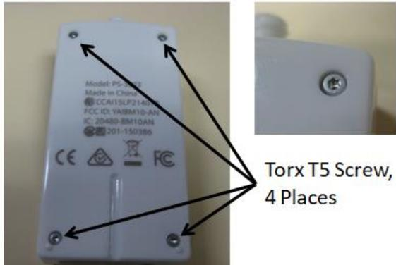
**Step 2:** Unscrew and remove the (4) Torx Screws with the T5 Screwdriver.
